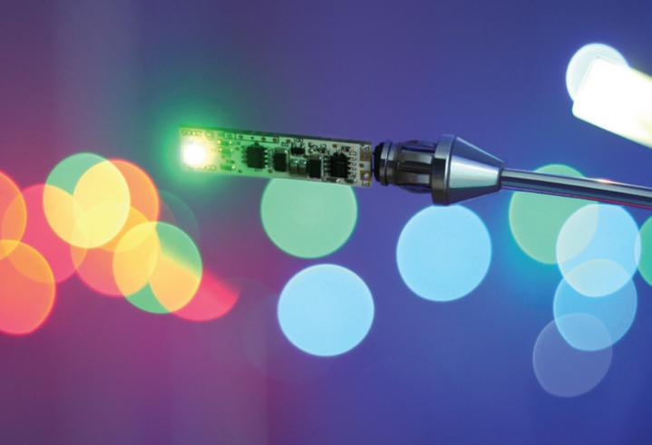
Benefits of using the ELS litebits over halogen globes include full colour control, as well as minimal power consumption, virtually no heat production, resistance to vibration and shock, with an expected service life of over 10 years.
